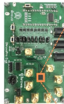
DhruvaPro Eval. Board • QFN 32 Package • 65 nm CMOS
