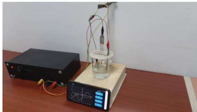
The chronoamperometry of 1 mM and 750 \mu M ferricyanide on a screen printed electrode by potentiostat and a commercial potentiostat
