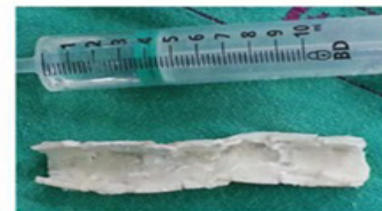
3D hydroxyapatite tray fabricated by using bone cement
