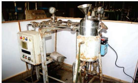
Hybrid Technology (Hydrodynamic Cavitation set up with pretreatment tank)
