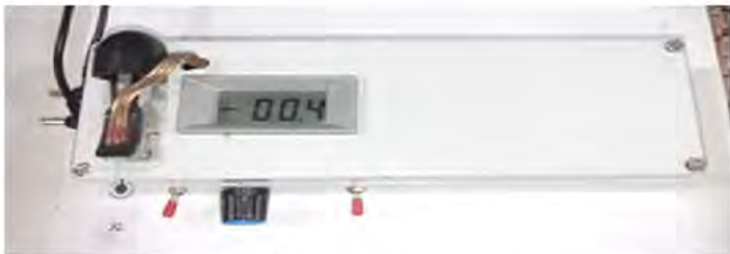
Biosensor device with display unit, Screen Printed Electrode connector clip, zero setting knob
