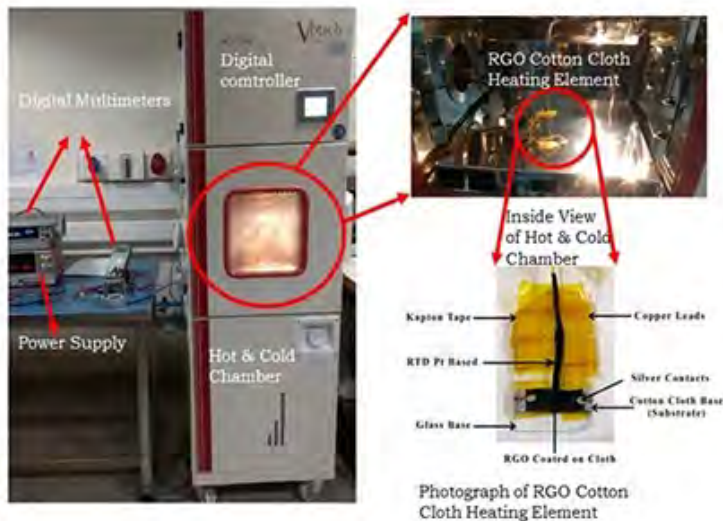
Experimental testing set up of RGO nanosheets Cotton Cloth based Heating Element maintained at different ambient temperatures and tested results.
