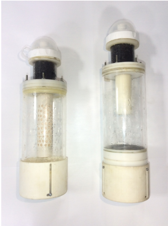
Water Purifier bottle prototype with (A) ultra-filtration (UF) membrane in packaged state, (B) micro-filtration (MF) membrane in expanded state
