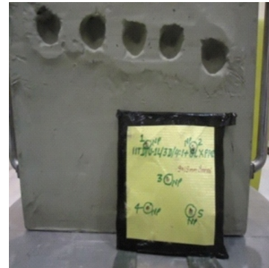
Backing material deformations after BFS test
