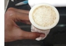
Topview of Hollow Fiber Membrane Bundle
