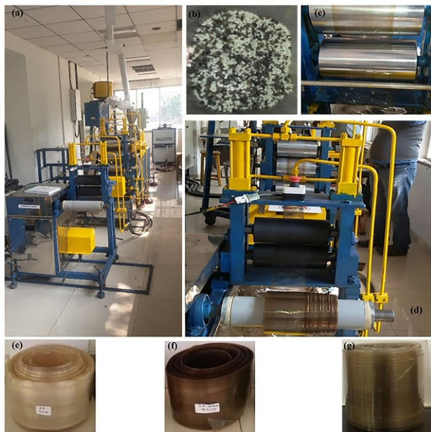
Figure: Pilot plant scale production of PLA grafted chitosan bionanocomposite films (a) Twin screw extruder for lab and industrial scale film processing, (b) PLA granules coated with grafted chitosan, (c) Bionanocomposite film passing through rotating drums, (d) Processing of bionanocomposite film, (e) Extruded PLA film, (f) Extruded PLA grafted chitosan bionanocomposite film and (g) Laminated PLA grafted chitosan bionanocomposite film.
