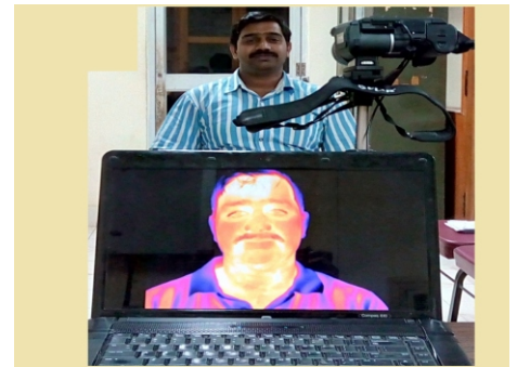
Setup for capturing facial thermal image using FLIR T 650 SC camera
