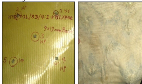
Face side (left) and back side (right) of STF treated fabric panel after BFS test
