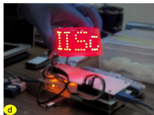
Fig1 (a). Flexible Display which shows the characters of institute name II Sc and dept., title as IAP.
