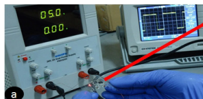
Fig2 (a). 555 timer circuit as an Astable Multivibrator. (b). Expanded view of the flexible circuit used for 60% duty cycle wave generation. (c). Tested and verified data Shift register circuit on a flexible substrate.
